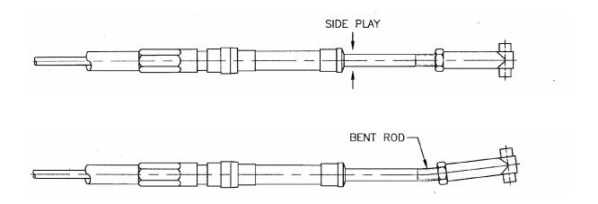
It is possible that a cable end may become bent either in transit during an installation or simply gets hit after it is installed. This, in fact, will also cause binding between the core rod and the sleeve.
