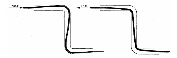
This is known as lost motion and it is impossible to eliminate lost motion in a push pull cable. In a good quality cable, however, it is kept to a minimum.
